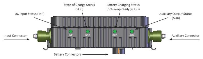
The Merlin-3™ SBC monitors and displays the status of the battery, input and output power availability via dedicated LED lights.
